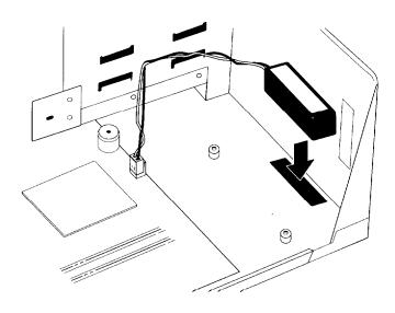
5. Connect the battery cable to connector CN3.
